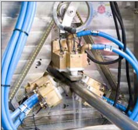
The STP-System works with three probe carriers (couplant wipers and protection housing of the system are dismantled in this picture). Each probe carrier holds one probe for normal incidence. Two angle beam probes can also be integrated in each probe carrier for detection of surface-near flaws.
