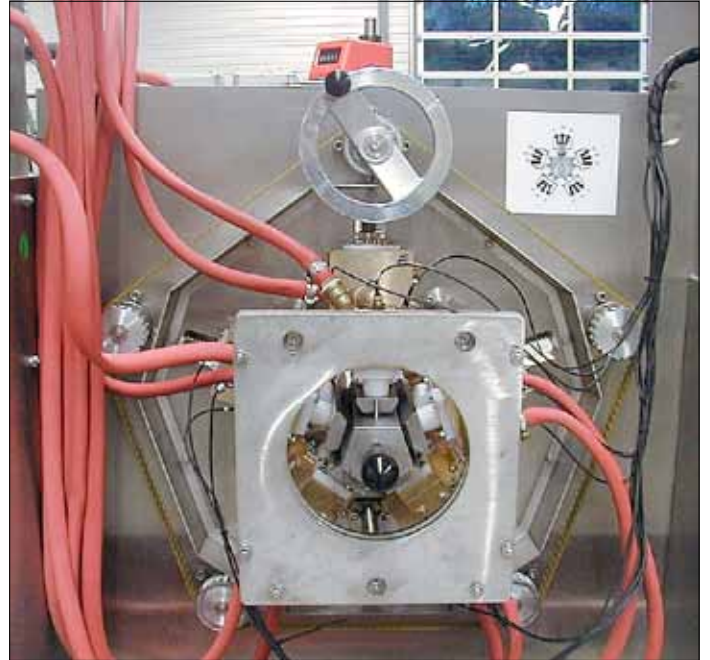
Testing mechanic with 15 probes for round bars (currently equipped with pentagonal calibration block)
