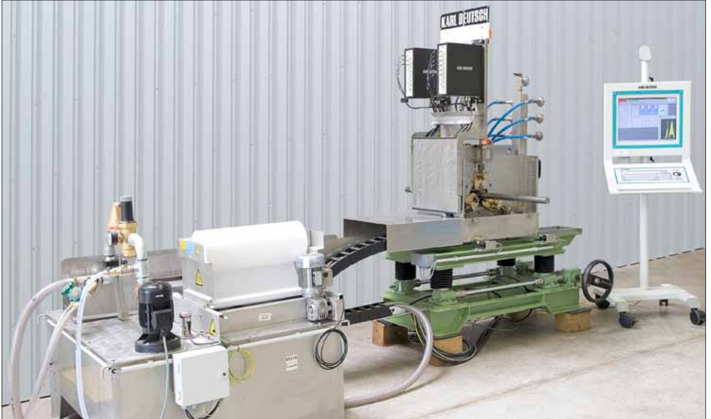
Bar testing system with water filter unit, test table and operator panel.
