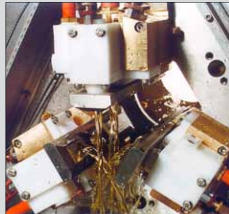
Detailed view of the probe carriers with water supply. The guidance on the bar surface is achieved with hardened skids.
