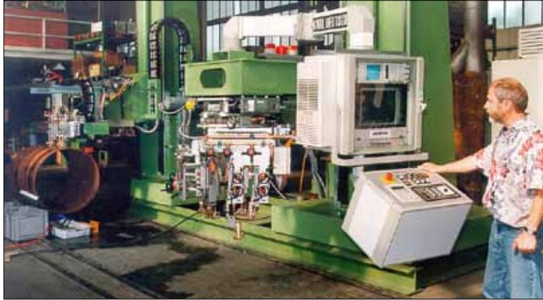
Testing system during assembly: The system consists of two separate machine stands, one for the weld inspection and a second stand for the strip (pipe body) inspection
