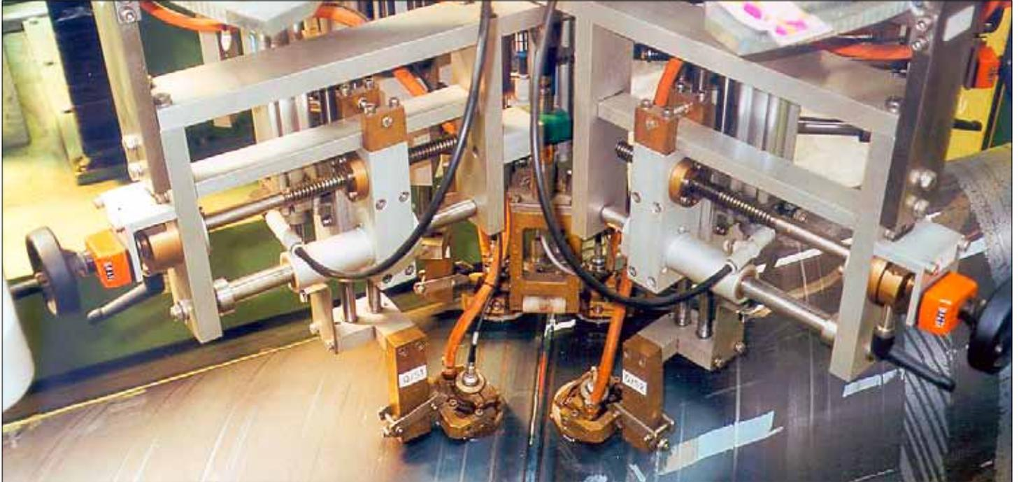
This photograph shows the probe holders being perfectly centered with respect to the weld. The seam tracking is carried out in an automated manner. The operator can observe the status of the seam tracking device by checking the illumination of a laser pointer. A red line can be seen on the weld crown.
