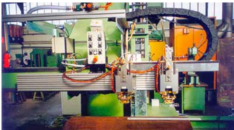
Mechanics for the oscillating strip inspection (pipe body test): The pipe is transported in a helical motion. The strip material between the welds is inspected with oscillating probes. The required coverage determines the number of probes (2 probes in the shown case).
