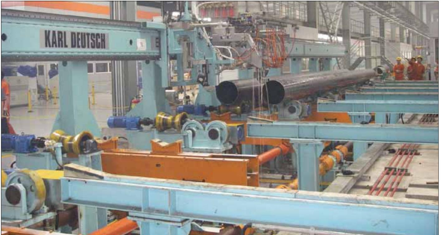
Testing Portal (Offline Testing Machine): Onsite operation with transverse conveyor for pipe feeding and linear discharging of the pipes. This machine was also equipped with two additional probe holders for the pipe end inspection.
