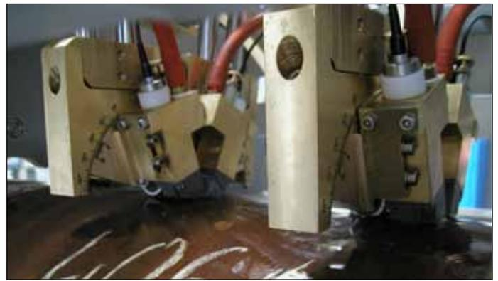
Probe holders with angular incidence for the detection of longitudinal defects. Stable ultrasonic coupling is achieved by water jet coupling (also called squirter technique). The incidence angle can be adjusted without steps for a perfect setting with respect to pipe diameter and wall thickness and without changing the probe.
