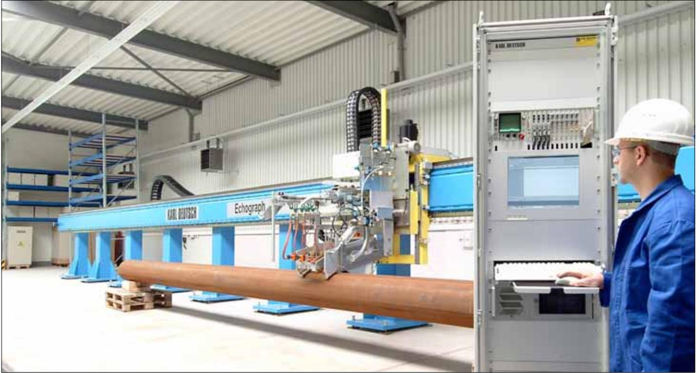
Testing portal (offline testing machine) during assembly at KARL DEUTSCH workshop
