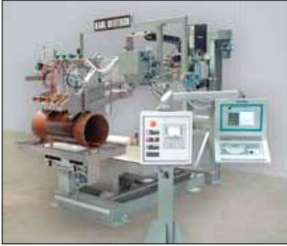
Online Testing System for ERW-Pipes. The probe holders can be moved between the testing position and the calibration position. In the calibration position, a short pipe segment is used for the sensitivity setting of all probes.
