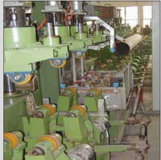
Examples for the helical tube conveyor which must provide a transportation of the tubes without vibration. The rotational and the linear tube speed must be perfectly adjusted for the respective tube diameter. The angles of the supporting rollers (below the tube) and the pressure rollers (above the tube) with respect to the tube axis are therefore adjustable.
