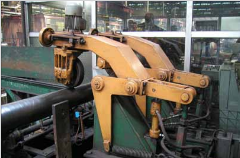
Examples for the helical tube conveyor which must provide a transportation of the tubes without vibration. The rotational and the linear tube speed must be perfectly adjusted for the respective tube diameter. The angles of the supporting rollers (below the tube) and the pressure rollers (above the tube) with respect to the tube axis are therefore adjustable.
