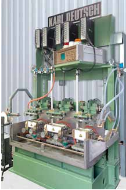
View of inspection system with three test chambers (longitudinal and transverse defects, wall thickness).
