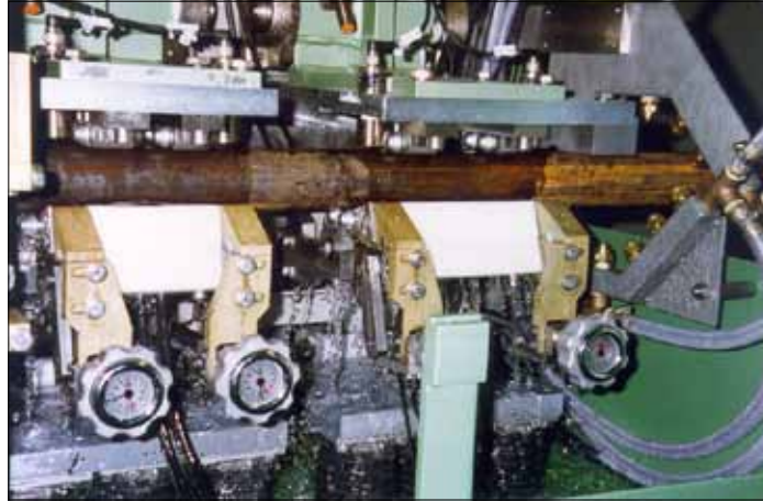
View of two test chambers for ultrasonic testing in partial immersion (probes below tube in water filled chamber). The shown testing system uses one chamber for the detection of longitudinal defects. The second chamber is used for transverse or oblique defects. The dials are used for adjusting the incidence angles of the ultrasonic probes.
