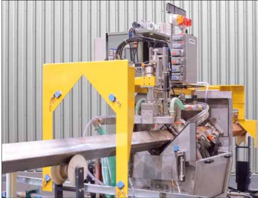
ECHOGRAPH-KNPS billet testing system
