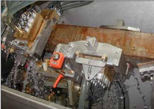
Four probe holders for quadratic billets, each carrier with seven probes and positioning from all four sides. The guidance is achieved by guiding rollers and hard-metal skids.
