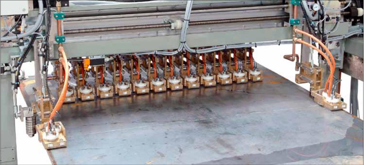
Narrow strips are fed through the inspection system in a centric manner. Only the probes above the strip are then active. The individual probe holders are pneumatically lowered into the test position. The end of the strip or largely damaged zones within the strip are automatically detected and the probes are lifted into the safety position.
