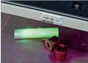
Inspection with the large area lamp under UV light
