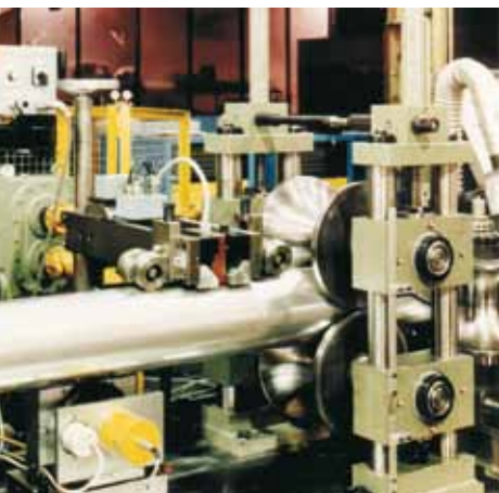
Weld seam testing with longitudinal magnetizing unit and segment coil
